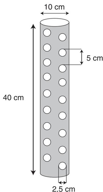
**Fig. 2** Schematic drawing of the pre-drilled push core used for sediment sampling in Kazan mud volcano.
